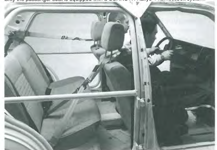
Only the passenger seat is equipped with a SCHROTH Rallye 4 harnessbelt system!
