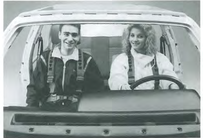
The driver seat is equipped with a SCHROTH Rallye 3 harnessbelt system with the tail strap installed at the C-pillar (anchor point "C").
