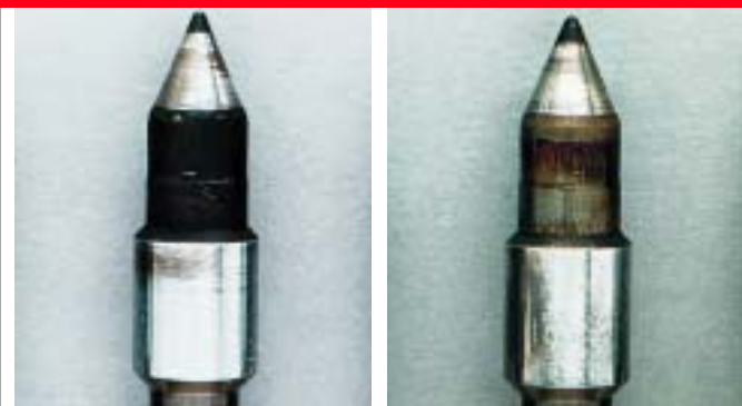
Injectors after 125 hours of Cummins L10 Injector Depositing Test using untreated diesel fuel and fuel treated with Diesel Kleen +Cetane Boost.
