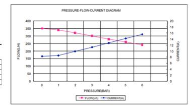
The factory fuel pump wiring may not be sufficient to handle the current draw of this fuel pump. Please update all wiring if necessary and add in a relay to ensure pump works correctly. If using the existing electrical plugs and wiring in vehicle ensure correct polarity is used on the new pump. If necessary, re-pin the existing one or use the included plug.
