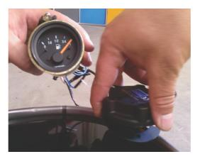
2. Insert the Fuel Level Probe into the Fuel Cell and refuel the cell until the fuel level reaches above the "Full Level" hole in shaft (see diagram).
